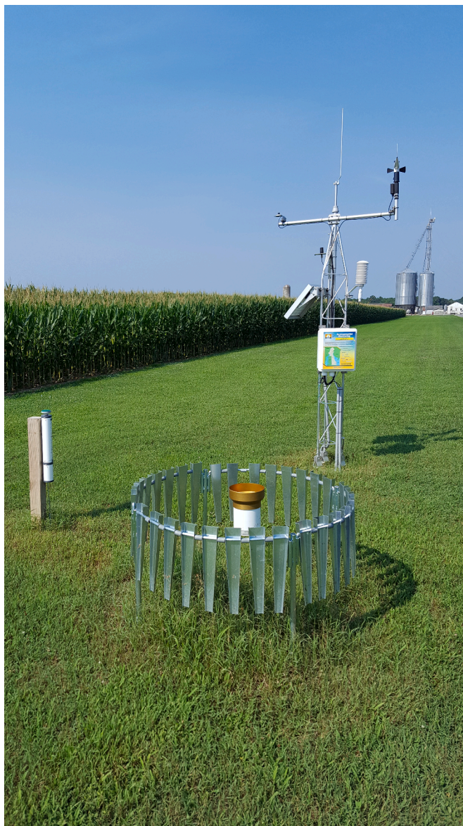
Fig. 2. Example of DEOS meteorological station used in this study (Station at Seaford, DE shown here). The atmometer (white cylinder object on the left) was installed similarly at each site - mounted to a 4 \times 4 wooden post approximately one meter high over a managed reference (grassy) surface.
