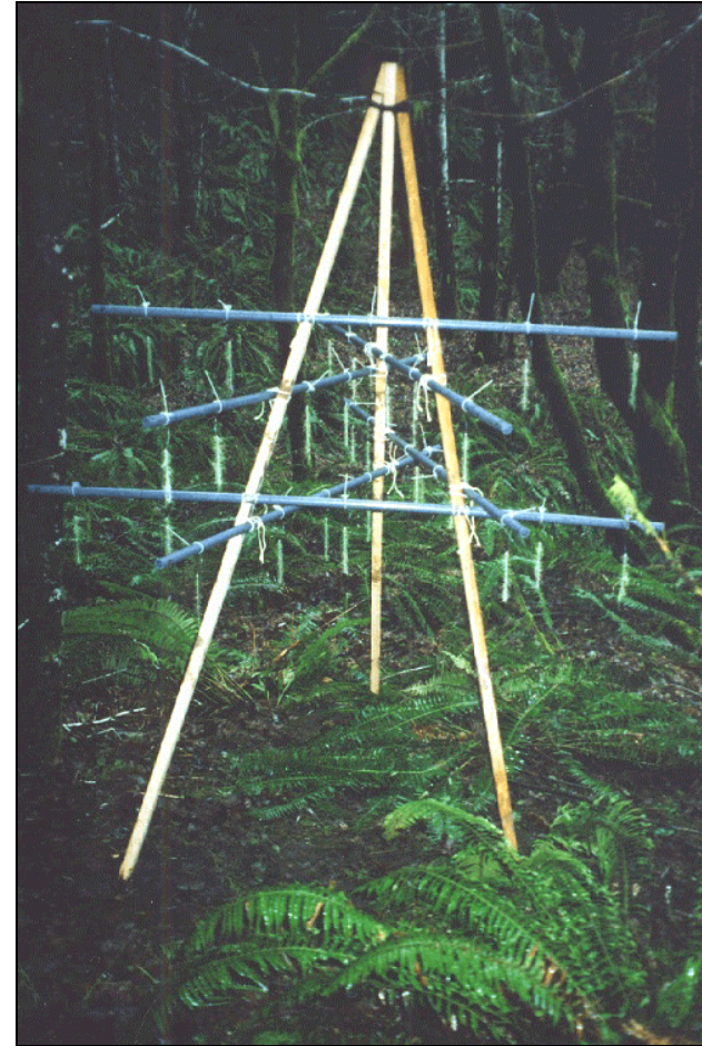
Figure 3.5 Tripod rack in place at a study site. Five transplants are suspended from each of the six PVC crossbars.
