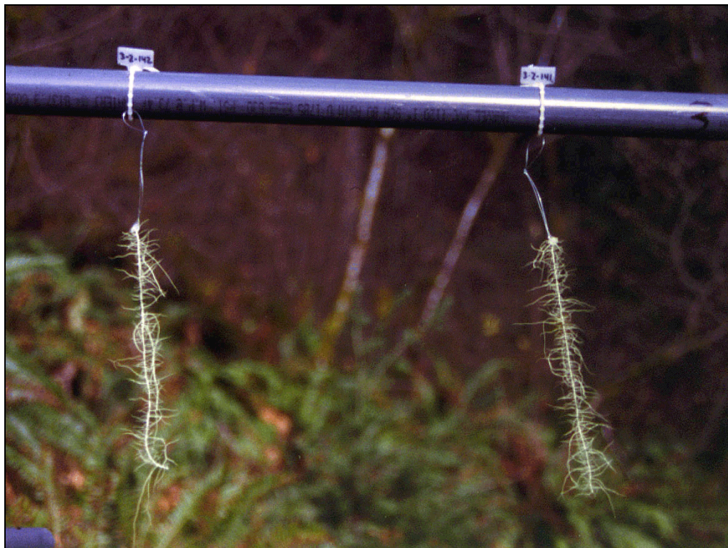
Figure 3.3 Usnea longissima transplants attached to PVC crossbars with releaseable zip ties.
